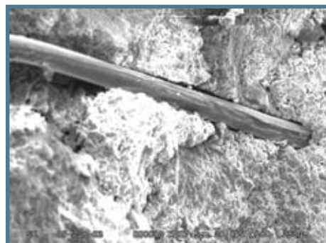
FIGURE A: Synthetic Polypropylene in Concrete (Note: Micro-voids around fiber and lack of paste/fiber bonding)
